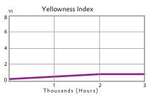
1/8" Nominal Thickness. Xenon arc per ASTM D 2565, Type B. Tested per ASTM D 1003.
